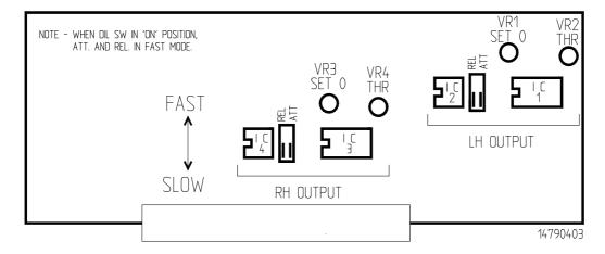
For correct tracking of the limiters when linked together, the DIL switch settings should be identical.
