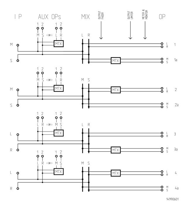
1a, 2a, 3a - a recording made in the M-S domain is ready for the application of all possible post-production techniques. This diagram also illustrates the manner in which it is possible to create an auxiliary output in the opposite domain from the main L-R output.
