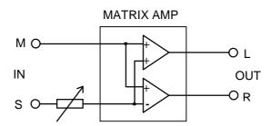
Increasing the S-signal widens the L-R stereo image; decreasing the S-signal makes the stereo image narrower.
