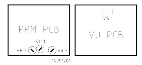
Main-output limiters - calibration involves two presets per output, to be found on the output module LH PCB. Using the 'L' output as the example...
